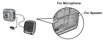
The external microphone input terminal does not correspond to an line level. Audio may be distorted when the line level is input. Audio distortion will be solved if you insert the following circuits. Under no circumstance should high level audio, such as from a speaker, be connected to this input terminal. Doing so is likely to damage the camera.
