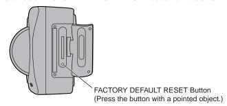
Pressing the FACTORY DEFAULT RESET button resets the camera to factory default. If you lose your user name and password, use this button to reset the camera.
